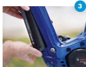
Push the top of the battery to detach it from the restraint support – the battery then drops into your hand
